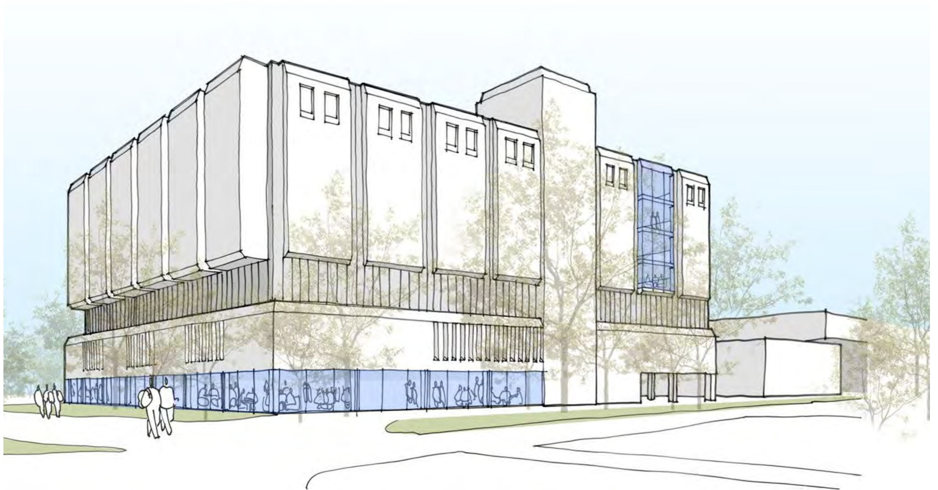
VIEW FROM SOUTH WEST, PHASE 3: GROUND FLOOR EXPANSION UNDER SOFFIT & GLAZED BAY OF NORTH-SOUTH 3RD-6TH FLOOR
